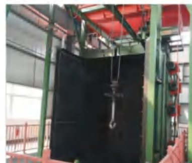
抛丸机 Q3750 (吊) [内腔尺寸: 3500x6000]
